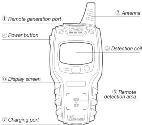
**Start:** press and hold the power button for 1 second
